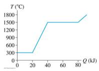
14. An experiment measures the temperature of a 200 g substance while steadily supplying heat to it. What is the specific heat of the substance during the liquid phase?
